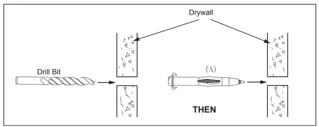
With a screwdriver, press down firmly and turn the bolt clockwise until the barrel crimps against the inside of the wall and the bolt starts to slip. Unscrew the bolt just enough to allow you to hang your item.
