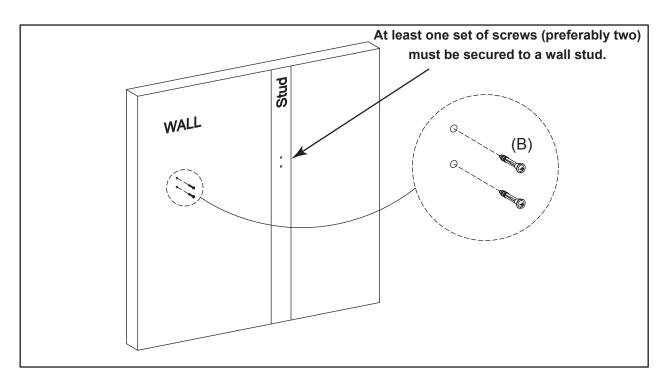
STEP 2: Use screwdriver to mount Bracket over marked locations on wall. Use Wood Screws (A) through Bracket into a stud and Expansion Bolts (B) into drywall. NOTE: At least two sets of screws must be mounted into a wall stud.
