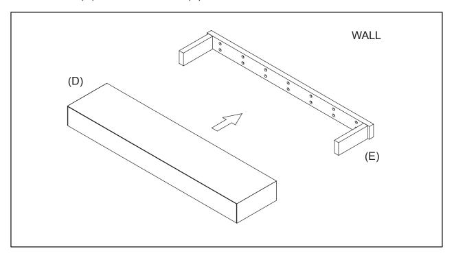
STEP 4: Using screwdriver, secure Shelf (D) to Bracket using Small Screws (C) through holes on underside of Shelf. Firmly secure.
