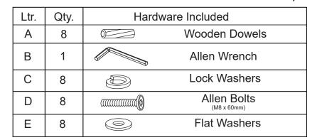
Hardware Packet located in top of shipping carton. (Parts A through E).
