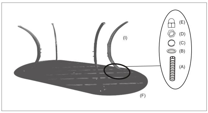
STEP 2: Loosely attach the Center Plates (G & H) to the Table Legs (I) by screwing in the Washers (B), Lock Washers (C), Nuts (D) and Nut Caps (E) from the inside of the Center Plates.
