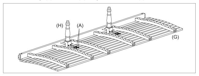
STEP 2: Attach the Wood Bolts (I) to the Legs (H) and Seat (G) using the Allen Wrench and 6 60mm Allen Screws (B).
