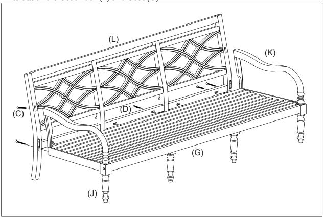
STEP 5: Insert the Screw Plugs (E) in the Screw Holes.
