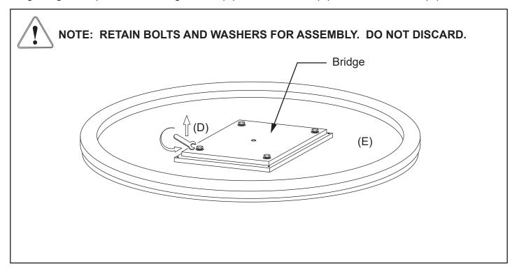
**STEP 2:** Set Base (F) upright. Align holes in Bridge with T-nuts embedded in top of Base. Replace Bolts (A), Lock Washers (B) and Flat Washers (C). Fully tighten using Wrech (D).
