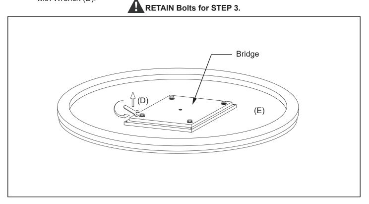
STEP 2: Align holes on the Bridge with hole in Base (F). Secure using Hexagonal Bolts (A), Lock Washers (B), and Flat Washers (C). Fully tighten using Wrench (D).
