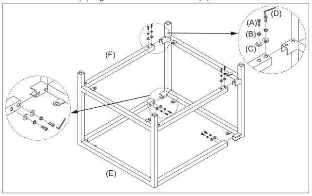
STEP 2: With the structure upside down, align the brackets on the Main Panels (E) to the Wood Top (G). Using Bolts (A), Lock Washers (B) and Flat Washers (C), attach the Wood Top and tighten with the Allen Wrench (D).
