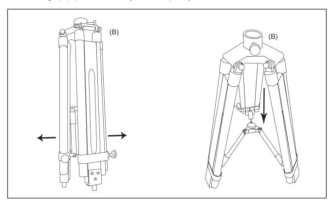
STEP 2: Slide the joint sleeves over the joint in the center to lock Legs (B) in place. Place the Table Top (A) onto the Table Legs and secure it by tightening the knob on the Leg base.
