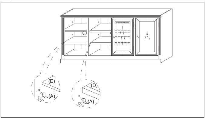
LEVELERS: If necessary, the Console may be leveled by adjusting LEVELERS located on the bottom of each corner which are accessible INSIDE the Console. Use a Flat Head Screwdriver to turn clockwise/counterclockwise to adjust. Cover holes with Wood Plugs (C) when complete.
