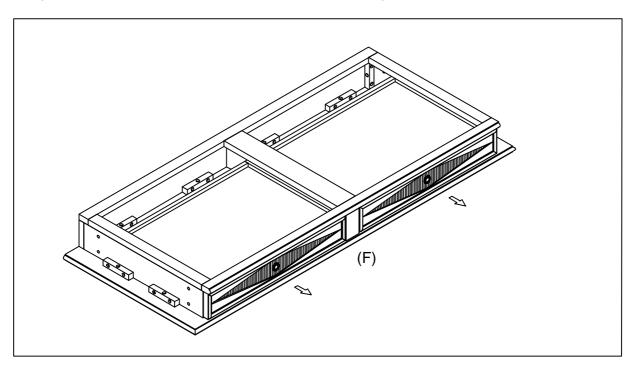
STEP 2: Attach the Legs (G) & (H) to the Desk Top (F) from the inside of the drawer holes using a Bolt (A), Spring Washer (B), and Flat Washer (C). Tighten using the Allen Wrench (D).
