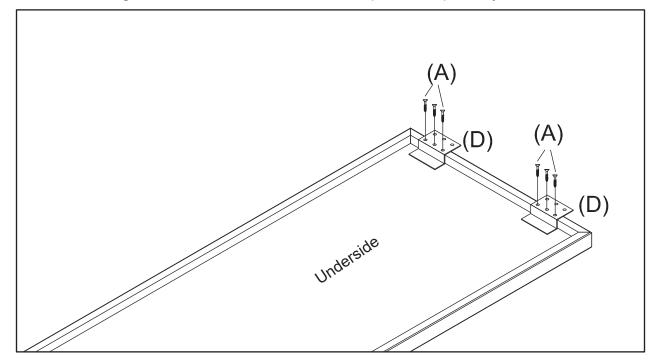
STEP 5: Attach Connectors (D) to underside end of each Original Home Office Top using Wood Screws (A). Firmly tighten.
