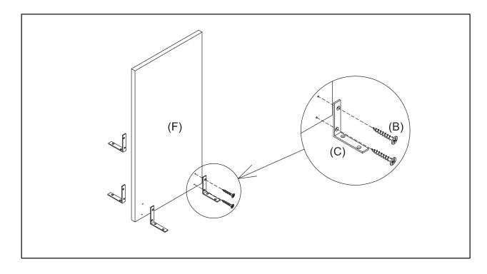
STEP 3: Invert Top (E) onto a clean, level, padded surface. Secure L-Brackets (C) on Leg (F) to Top (E) using Coarse Wood Screws (B).
