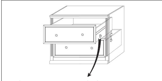
**NOTE:** To prevent accidental tipping of the Console, both drawers are equipped with safety locks which permit only one drawer to be open at a time.
