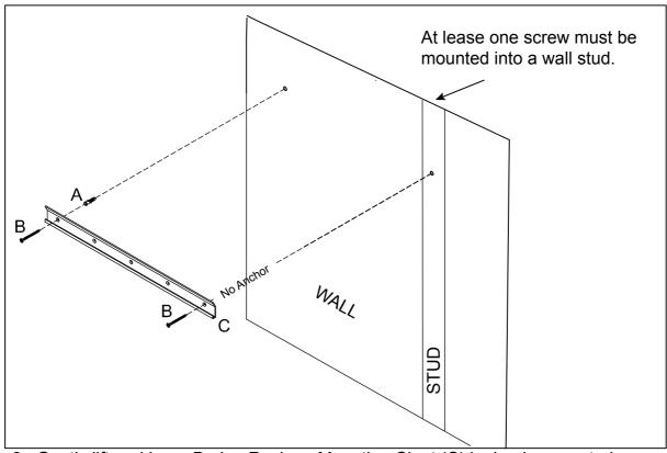
Step 3: Gently lift and hang Drying Rack on Mounting Cleat (C) by hooks mounted on each end of the Drying Rack.
