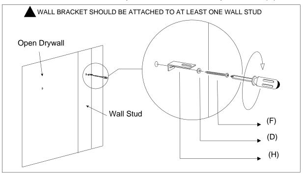
STEP 4: For Bracket (I) location in Open Drywall, first use a 5/16" bit and drill a small pilot hole. Next, use a Hammer to GENTLY tap in Expansion Bolt (H) until Teeth sink evenly into wall surface,
