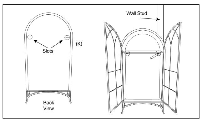
STEP 2: Position Cabinet (K) in location for intended use and check for level. Cabinet is equipped with Rotary Levelers located under each corner. If necessary, Cabinet may be adjusted by carefully lifting applicable corner and turning Leveler clockwise/counterclockwise. NOTE: Check marks from STEP 1 and redraw if Cabinet has moved up or down during leveling process.
