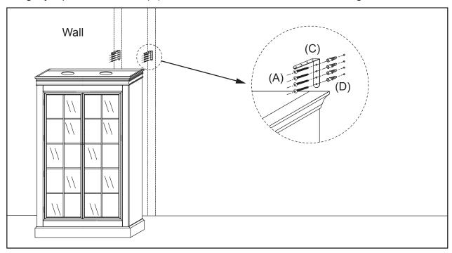
STEP 6: Slide the Cabinet underneath the previously installed L-Brackets (C) and use 2 or more of the Long Screws (A) to attach the L-Brackets to the Cabinet with a screwdriver.
