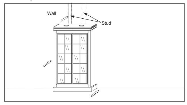
STEP 4: Slide the L-Bracket (C) over the top corner of the Cabinet and in front of the previously marked stud. Mark the wall at the top of the L-Bracket.
