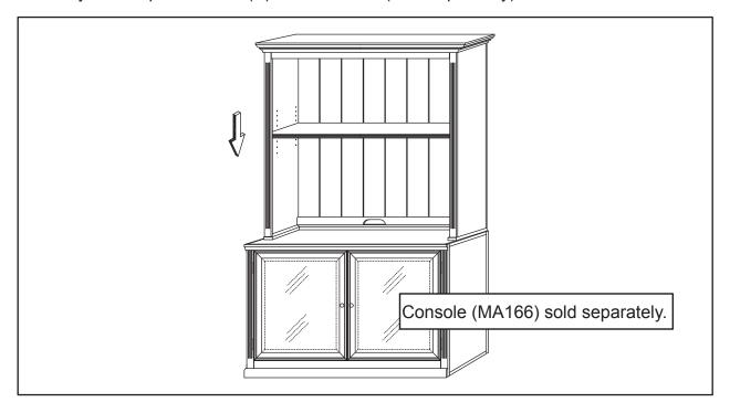
STEP 2: Align Connecting Plates (B) and attach to base of Hutch (E) and top of Console using Screws (C). Firmly tighten using Phillips screwdriver.
