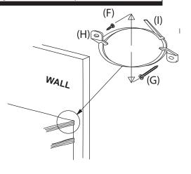
Attach a Bracket (H) to back of unit using a Small Screw (F) through smaller hole. Using a Large Screw (G), attach the remaining Bracket to wall into a wall stud approximately 2 inches lower than Bracket on unit. Push unit to wall, align brackets vertically, then attach together using Retention Belt (I). Be certain Belt is secure and unit is safe from tipping forward.
