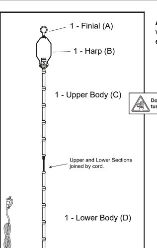
**ASSEMBLY:** Carefully pull Cord through Lower Body (D) while bringing Upper Body (C) together. Insert threaded and turn clockwise to tighten
