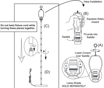
**INSTALL BULB:** 3-Way Socket rated up to a 100 Watt Type A (E26-Medium Base) bulb. LED recommended. To mimic an incandescent, choose 2700K Soft White.
