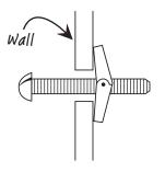
As with wall anchors, installation begins with drilling a pilot hole and then lightly tapping the toggle bolt into position. Good for heavier jobs, toggle bolts have spring-activated "wings" that fold out once inside the hollow wall. As you tighten the bolt with a screwdriver, the wings expand and are drawn against the wall. Note: Once installed, removing the bolt from the wall will cause the wings to detach and fall behind the wall.
